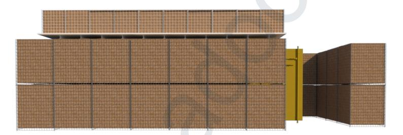
MAdoorS, often simply referred to as "Kumkoy barriers" or "Kumkoy bunkers," are a type of protective structure made from wire mesh containers filled with soil, sand, gravel, or other locally available filling materials. These structures are commonly used for military fortifications, flood control, erosion prevention, and other applications where rapid construction of protective barriers is required.
