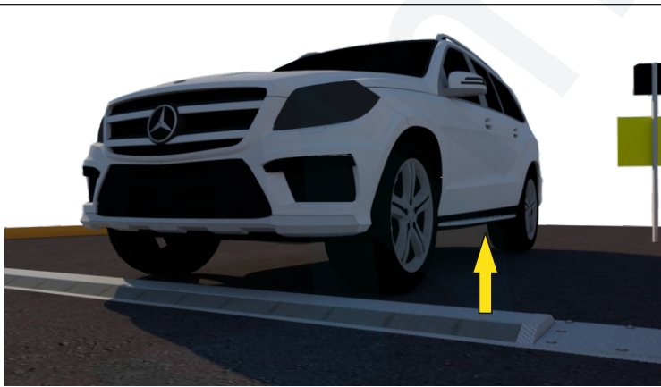
A. If the set speed limit is exceeded, the automatic speed bump will rise in the direction of the arrow.
