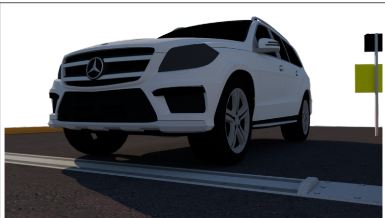
B. If vehicle cruising at the speed limit in accordance with the rules, the hump will not rise from the ground
