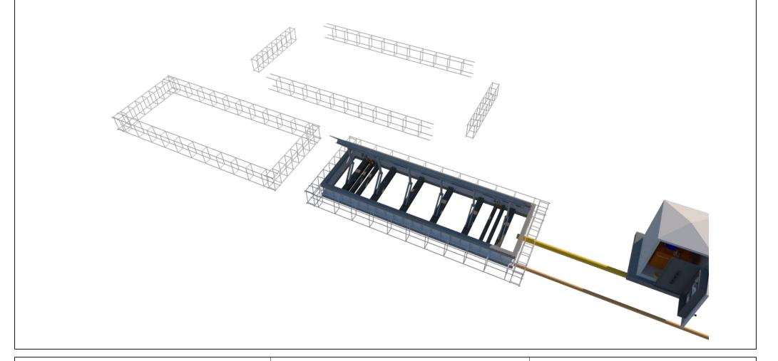
Shallow Mounted Road Blocker Construction
