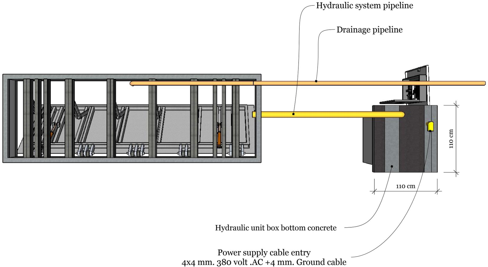
Shallow Mounted Crash Rated Wedge Road Blocker Barrier System
